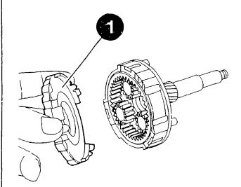
Checking planetary gear train
